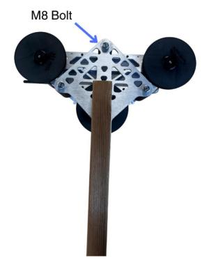
Feed the paracord or cable through the line and reinstall the M8 bolt and spacer.
